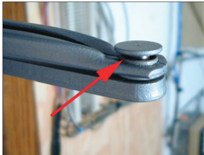
12. Another point in the arm assembly that has a lot of tolerance.
